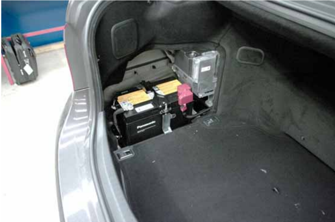
12v Batteries are located in the boot of all hybrid models. The isolation plug will also be in the boot except for the RX 400h where it is located below the seat in the nearside rear passenger door.
