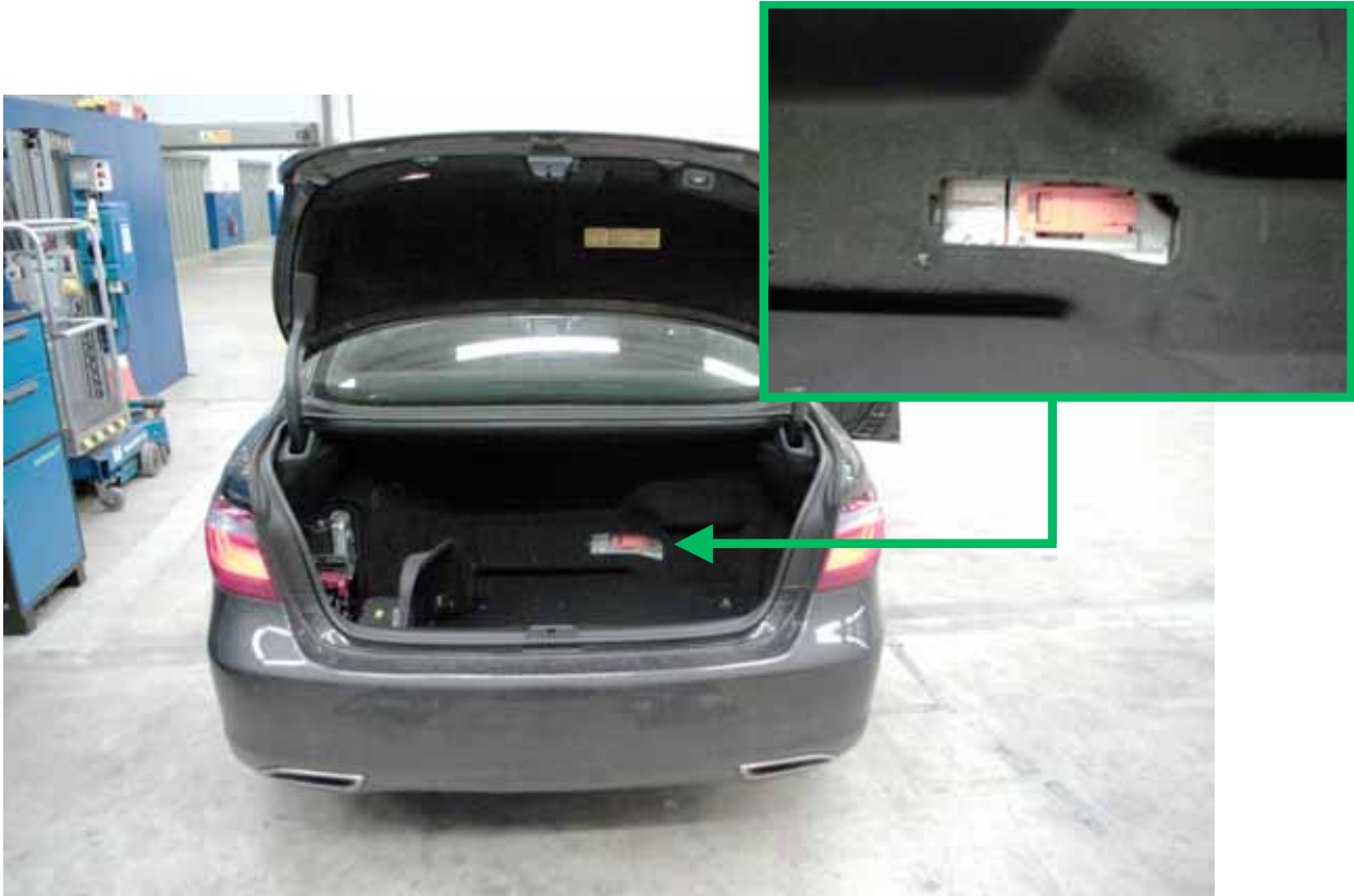
12v Batteries are located in the boot of all hybrid models. The isolation plug will also be in the boot except for the RX 400h where it is located below the seat in the nearside rear passenger door.
