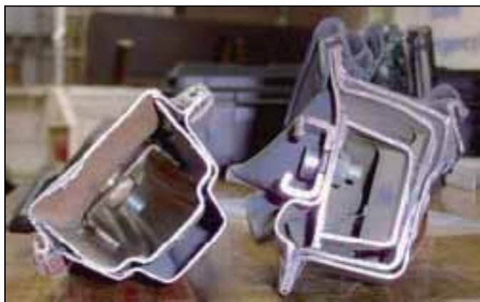
Old style B Post an Newer Style B Post with UHSS Inserts
